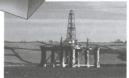
Oil and natural gas can be extracted by drilling into a reservoir and pumping the contents to the surface. Many large reservoirs are found offshore, along the continental shelves. Special drilling platforms can be towed out by boats and anchored the reservoir.
